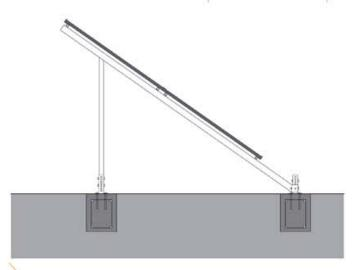
The fixation of the panels to the metallic shapes and the laying of the electrical cabling are carried out in a rapid, simple and economic way, so the aluminum shapes come with some holes for the fixation of the screws and it is possible to make this in any point of the metallic shape. In addition the top metallic shape where the panel lies, possesses a place where to put the electrical cabling, which reduces the time of the laying the electrical cabling.
